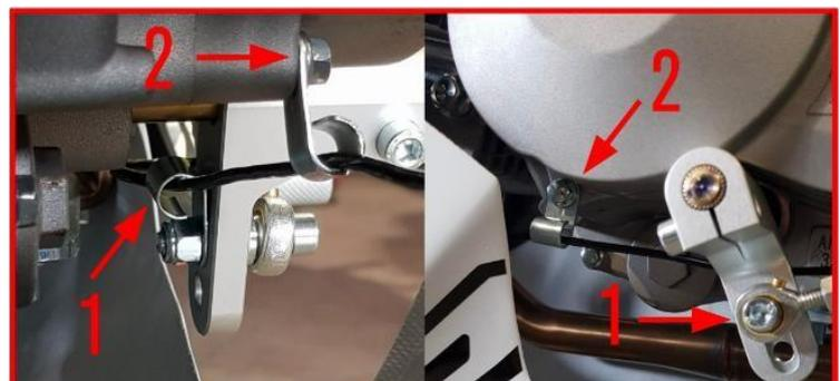
**5** For a correct fixing of the wire use the fairlead included in the assembly kit. Position the fairlead "1" behind the gearshift arm and the fairlead "2" on the stator cover. (This procedure is the same for Ohvale GP-0 and Ohvale GP-2)
